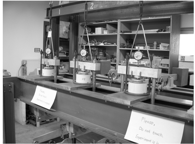
Fig. 3. Loading Section Based on Leverage Mechanism
