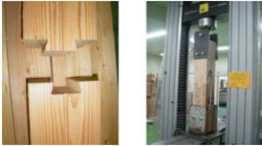
Fig. 2. Tested dovetail joint and testing.
