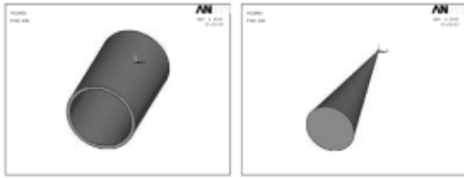
Fig. 1. Cylinder type and cone type element of knot model for the compressive member.
