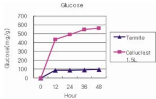
Fig. 6. Change of hydrolysis rate of glucose with reaction time by the enzyme from test termites (Substrate concentration : Cellulose 3%).
