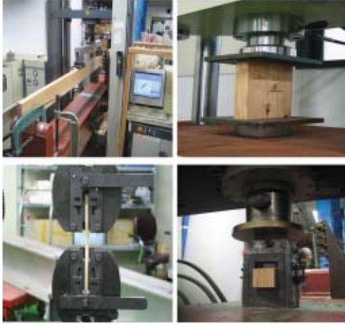
Fig. 2. Images of the strength tests (from left to right, bending, compressive, tensile and shear strengths).
