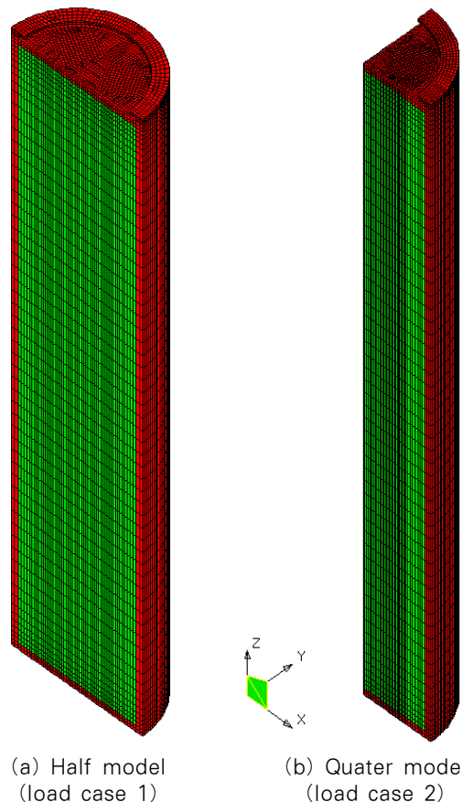
Fig. 4 Finite element model of the PWR canister (rotating angle(θ)=30°, diameter(D)=102cm)
