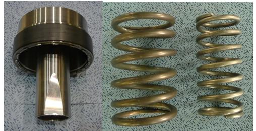
Fig. 3 Photo of the damper housing and springs
