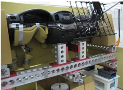
Fig. 4 BSR measurement system for vehicle interior module
