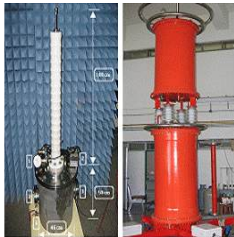
Photo 1. The Experimental Model GIS and AC 300[kV] Power Supply
