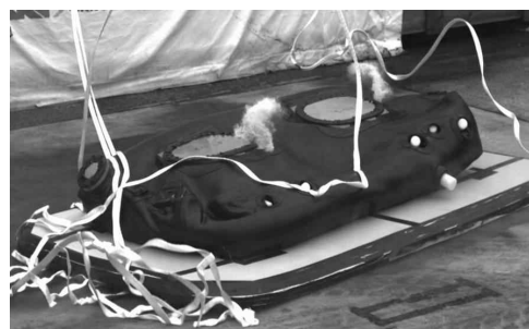
Fig. 11. Leakage by Damage of Fuel Tank in Crash Impact Test
