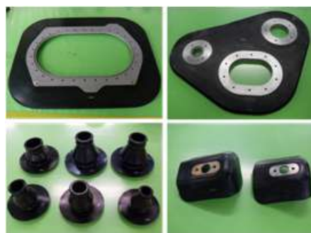
Fig. 3. Fittings of Fuel Tank
