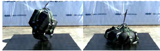
Fig. 1. Crash Impact Test for Verification of Material(Phase I Test)
