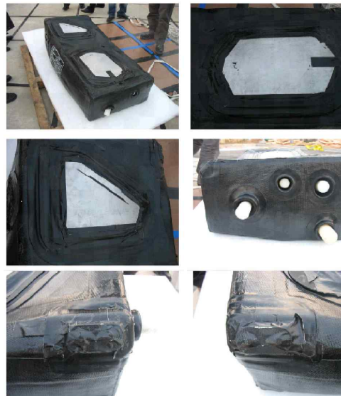
Fig. 16. Leakage Inspection of 2nd Crash Impact Test
