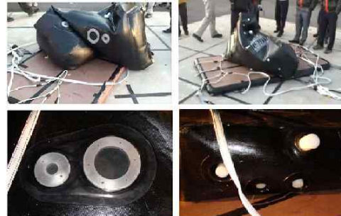
Fig. 15. Leakage Inspection of 1st Crash Impact Test
