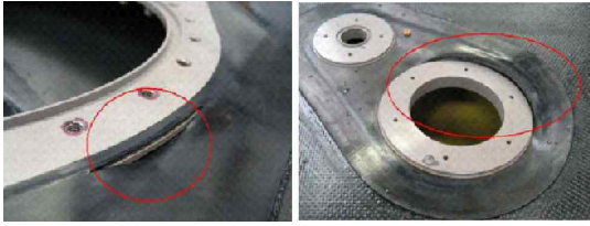
Fig. 12. Ruptured Fitting Area by Crash Impact Test
