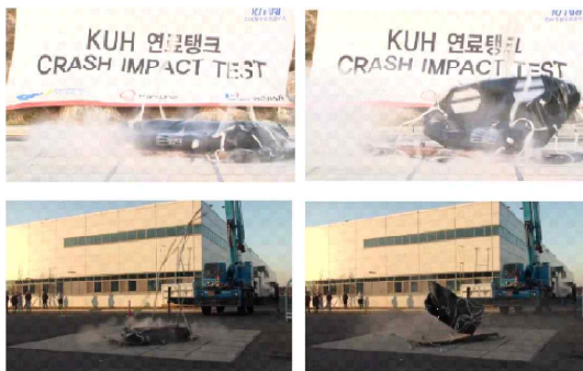
Fig. 13. 1st Crash Impact Test of Fuel Tank
