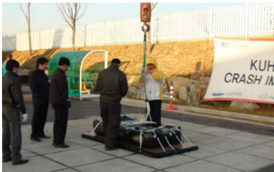
Fig. 7. Step 1 & Step 2 : Water-feed and sealing
