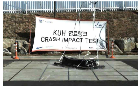
Fig. 10. Step 6: Onset of Crash Impact of the Fuel Tank
