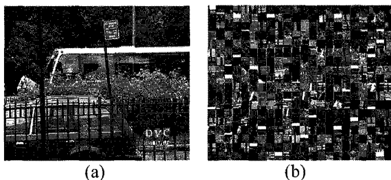
Fig. 6. Reconstructed images with and without deshuffling key: (a) with the correct deshuffling key, (b) without deshuffling key.
