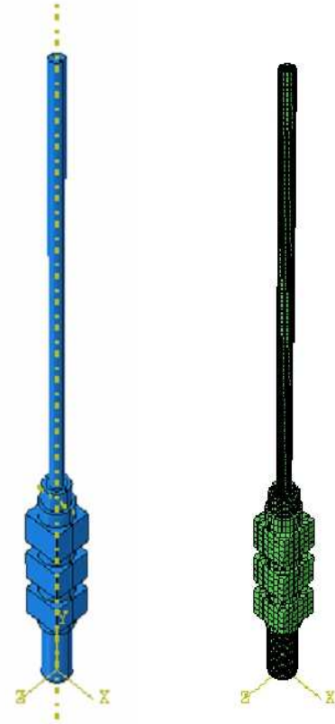
(a) 3D solid model (b) 3D solid FE model
