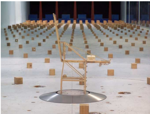
Fig. 4 Container crane model used for wind tunnel test
