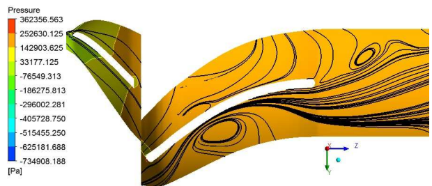
Fig. 9 Pressure contour and the stream lines on the 10% span of the scaled-down model at a design point
