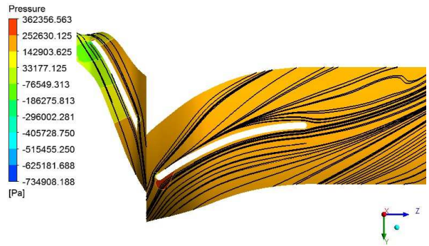
Fig. 7 Pressure contour and the stream lines on the 90% span of the scaled-down model at a design point
