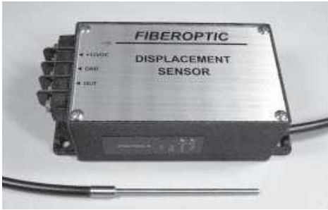
Fig. 3 Fiber Optic displacement sensor used in this study (PHILTEC.INC, USA, Model RC-60, \phi 5\text{mm} )
