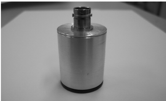
Fig. 8 Fabricated 500 kHz non-contact ultrasonic transducer.
