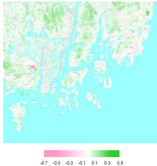
FIGURE 5. The NDVI image difference between 2000 and 2002 Landsat data over the study area. The green color bar means increased NDVI value than previous value, and the red color bar means decreased NDVI value during the comparison periods
