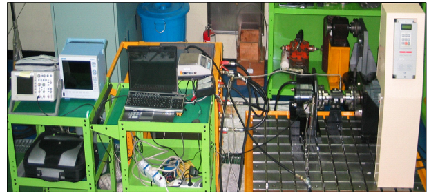
Fig. 8 Photo of test apparatus for radial piston pump
