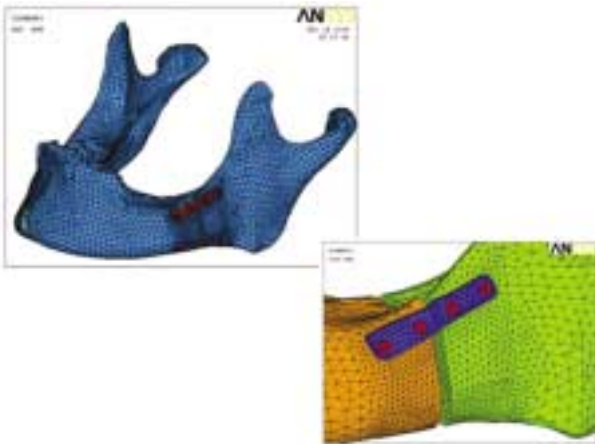
Fig. 6. Diagram of Type I model. Titanium plate is fixed to superior border of the mandible.
