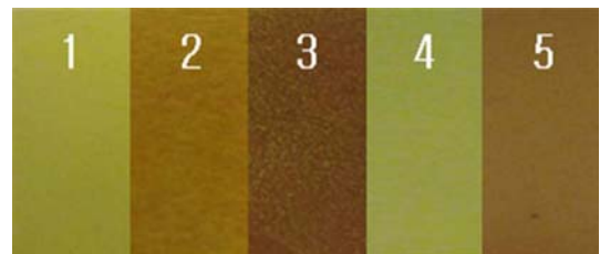
Fig. 1. Results of picrate method on the code of health/functional foods. 1; Sample A, 2; Sample A+0.01 mg KCN, 3; Sample A+0.1 mg KCN, 4; Sample A+250 mg amygdalin and 5; Sample A+250 mg amygdalin+0.01 mg KCN.
