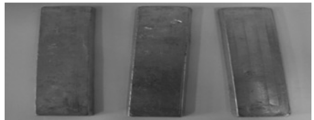
Fig. 2. The low melting alloy with bismuth(Bi) and tin(Sn).
