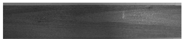
Fig. 4. Juglans mandshurica impregnated with low melting alloy.
