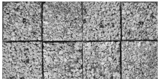
Fig. 6. Permeable polymer pavement block using polypropylene fiber.
