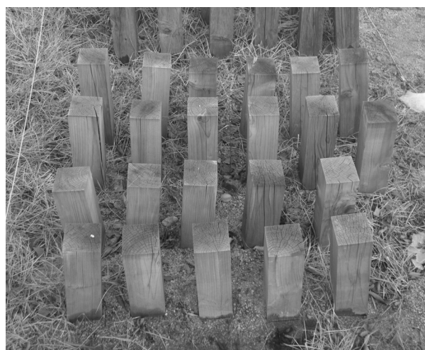
Fig. 1. View of the CCA-treated wood structures used in the experiment.
