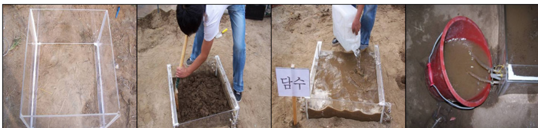
Fig. 1. The drainage after flooding method.
