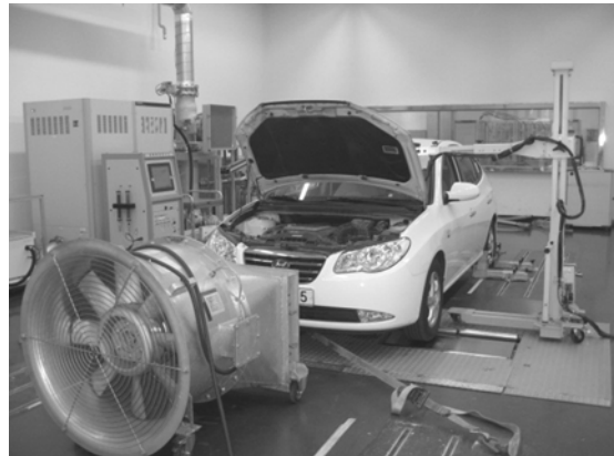
Fig. 4 Experimental setup of chassis dynamometer test for vehicle emission measurement
