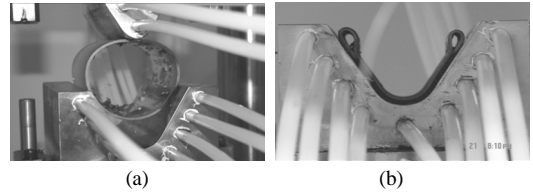
Fig. 2 Hot Press Forming Process: (a) heated blank starting to form and (b) quenched and unloaded blank
