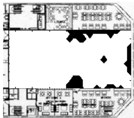
Fig. 19 Overview of area not satisfying the performance criteria, t=899sec, 6 x 4 m 2 /s
