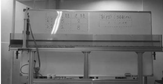
Fig. 2 Internal wave apparatus with removable gate
