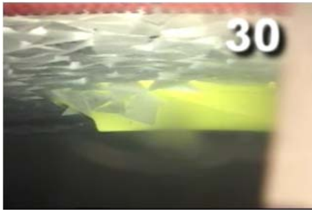
Fig. 14 Under water view of resistance test with pack ice (0.4m/s, 90%, \phi = 30^\circ )
