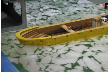
Fig. 8 Pack ice test of icebreaking cargo vessel in IOT ice tank
