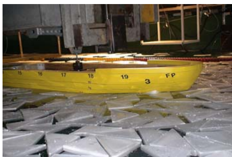
Fig. 6 Profile of resistance test with synthetic ice
