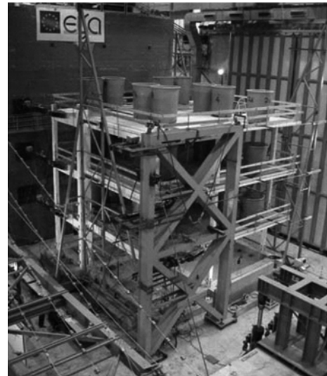
Fig. 12 Pseudo-dynamic test setup of the example frame
