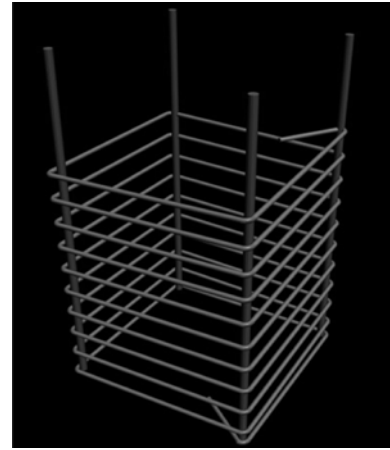
Fig. 3 Rectangular spiral reinforcement
