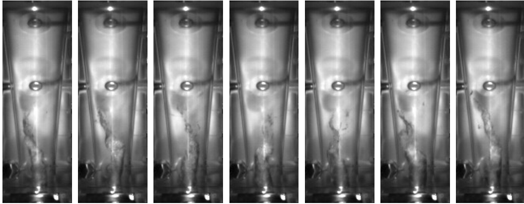
(a) Time interval = 0.00222 s; precession frequency 90 Hz ( St=5.054 )
