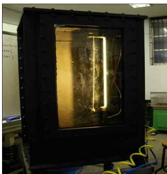
Fig. 3. Vacuum chamber for thermally-induced vibration test (500 width x 600 depth x 1200 length in mm)
