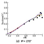
Fig. 10. Spanwise sectional thrust loading distribution on main rotor blade
