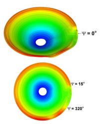
Fig. 11. Sectional thrust contours for one revolution of main rotor
