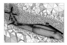
Fig. 7. Computational mesh for UH 60 configuration
