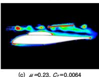
Fig. 6. Instantaneous vorticity contours at the fuselage symmetric plane for blades aligned along  $\mathcal{V} = 0$ °
