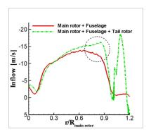
Fig. 9. Inflow distribution along  $\Psi = 0$  ° one chord length above rotor disk plane
