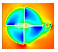
Fig. 8. Inflow contours at one chord length above rotor disk plane
