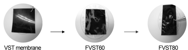
Figure 2. The visible change of the membrane according to the fluorination time.
