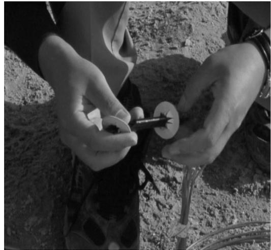
Fig. 3. Detonating fuse and electric detonator
