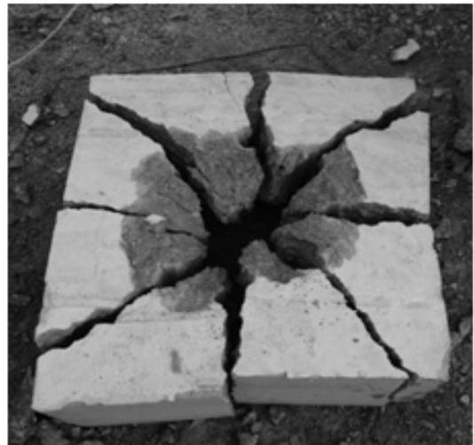
Fig. 5. Fractures of Type II specimen (weight of charge=10 g)
