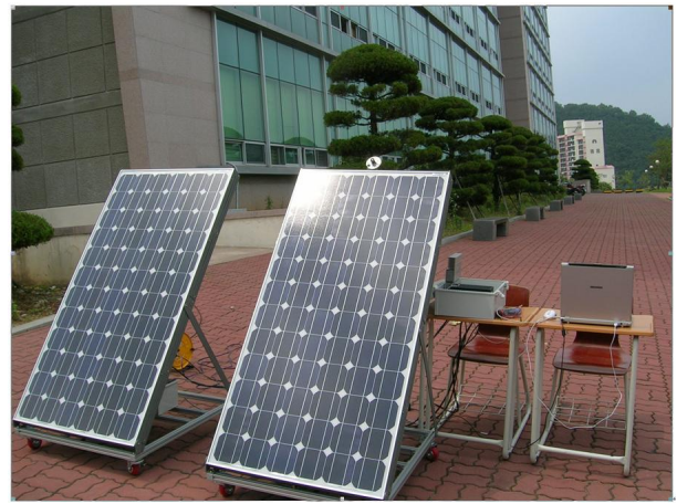
Fig. 8. Cooling experiment equipment of BIPV.
