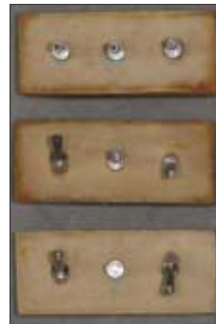
Fig. 2. Definitive casts with guide pins connected to show the angulation of the implant analogs. Top: parallel, middle: 30 degrees, bottom: 40 degrees.
