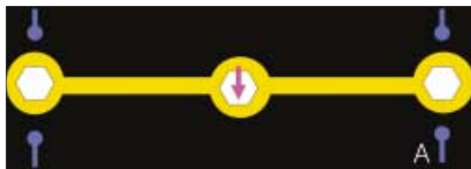
Fig. 5. Schematic drawings of the position and direction of measurement for statistical analysis. The arrows represent the screw tightening position and the round arrows represent measurement positions. A: Screw tightening of center analog and measurement of outer analogs, B: Screw tightening of left analog and measurement of right analog; screw tightening of right analog and measurement of left analog.
