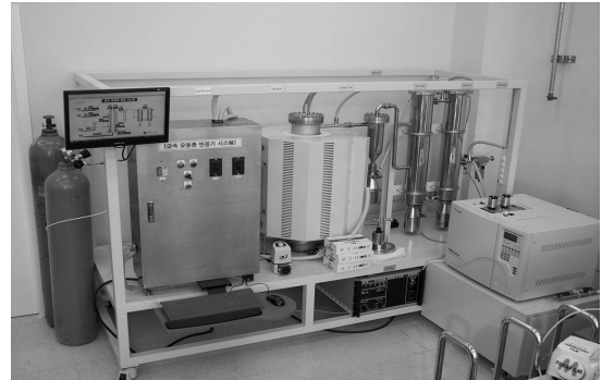
Fig. 1 Photograph of the fluidized bed pyrolysis gasifier: The main experimental apparatus consists of the pyrolysis reactor, heater, cyclone, double jacket separation and gas chromatograph.
