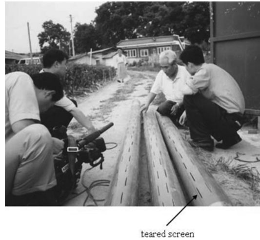
Fig. 7. Inflow of contaminated groundwater into groundwater well due to teared screen.
