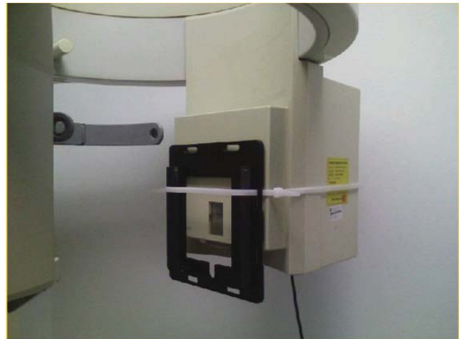
Fig. 2. Ionization chamber of DAP meter located at the tube side of cephalometric X-ray machine for DAP measurement.
