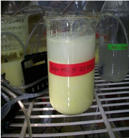
Fig. 1. A Sulfur master culture reactor (SMCR) and schematics of the sulfur toxicity monitoring system.
