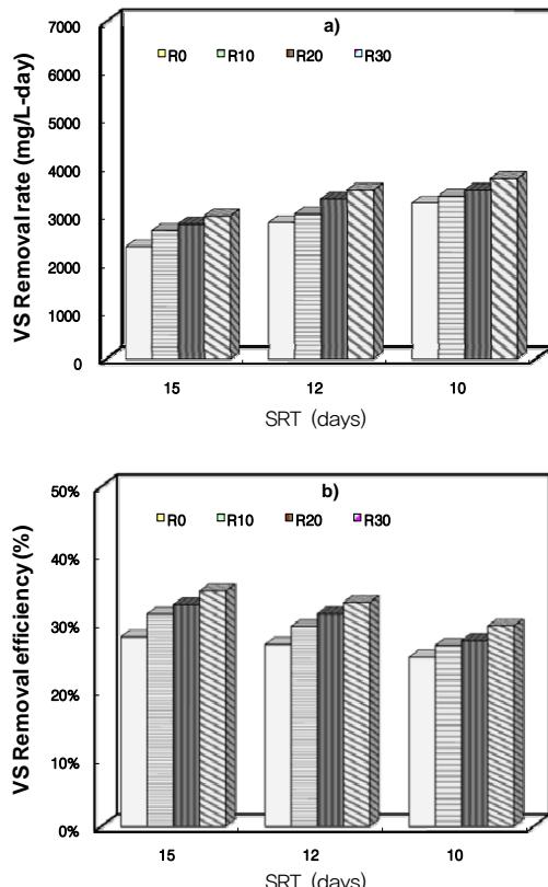
Fig. 3. VS removal at various pre-treatment time and SRTs; a) VS removal rate and b) VS removal efficiency.
