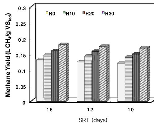
Fig. 4. Comparison of methane yield under different pre-treatment times and SRTs.
