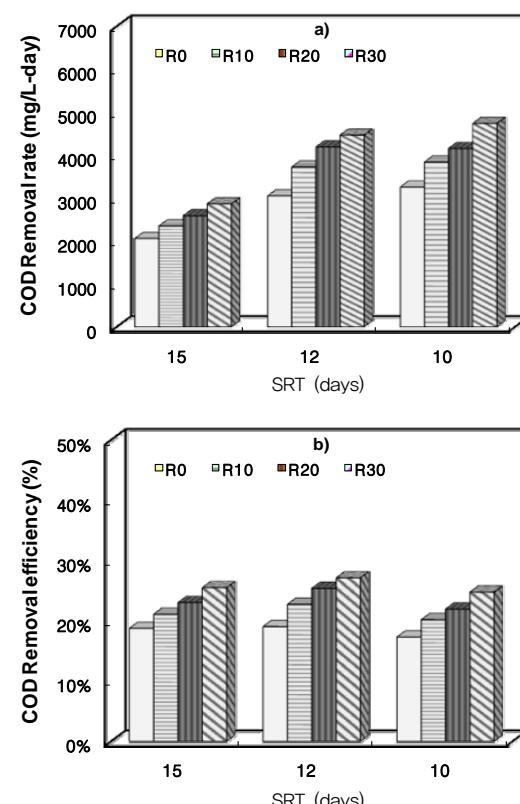
Fig. 2. TCOD removal at various pre-treatment time and SRTs; a) TCOD removal rate and b) TCOD removal efficiency.
