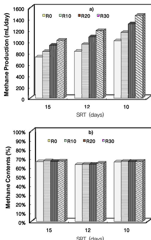
Fig. 1. Methane production at various pre-treatment times and SRTs; a) methane production and b) methane contents.
