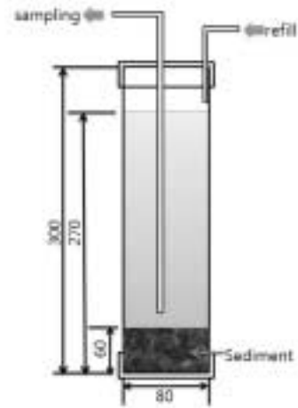
Fig. 3. Schematic diagram of apparatus used for release experiment.
