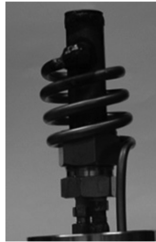
Fig. 3. Schematic diagram of flame calorimeter part(a) and shape of combustion chamber and heat transfer pipe(b).
