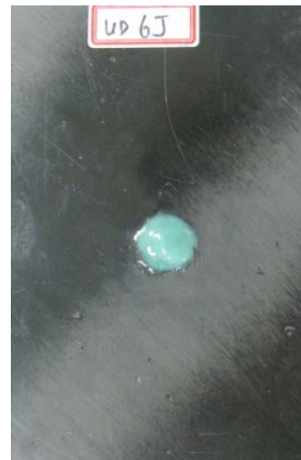
Fig. 9 Application of adhesive on removed area.
