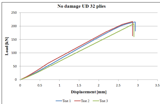
Fig. 11 Load-displacement curves of compressive test without damage.
