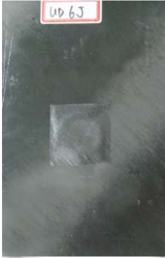
Fig. 10 Application of external patch.
