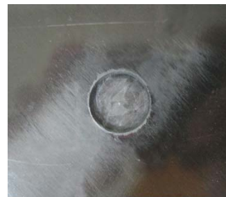
Fig. 8 Removal of impact damaged zone.
