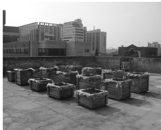
Fig. 1. The overall view of the experimental green roof systems with different soil types and depths on the rooftop.
