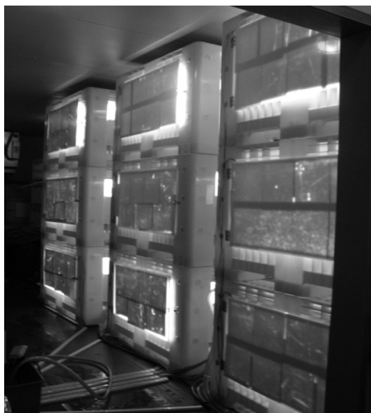
Fig. 1. Nine multi-purpose transplant production modules with fluorescent lamps as artificial lighting sources used in the present study. The modules were placed in a closed system.
