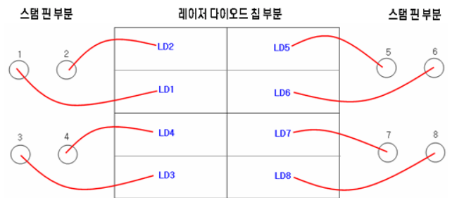
FIG. 9. Wire bonding of the laser diode chip and stem pin.
