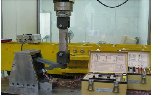
Fig. 20. Test Set-up for Full Scale Fatigue Test
